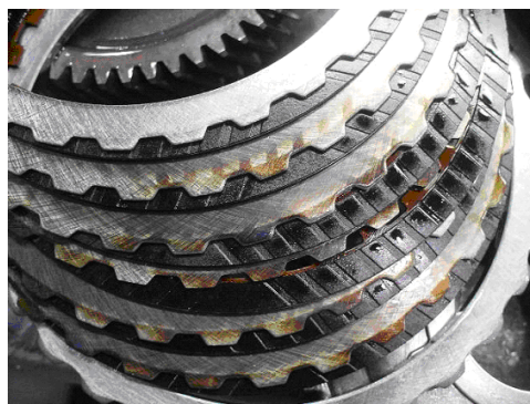
Burnt automatic transmission clutches
