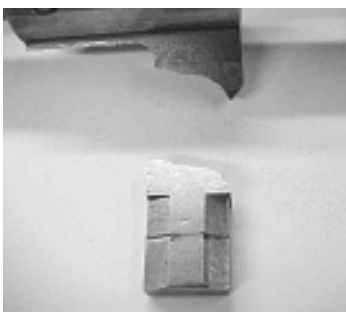
6-Speed 1-2 Shift Interlock Arm Broken
