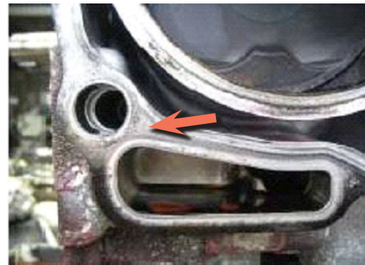
Rubber coating residue on oil sealing portion
